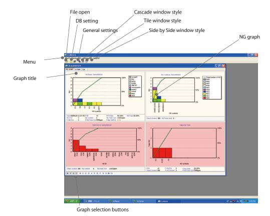
Window has a large graph area (you can swith NG Gragh, XY Shift and Cpk by tab), menu and tool buttons.
